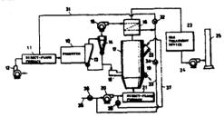
An incinerator for combusting sludge or the like is supplied with combustion air which is mixed with 5-40% by weight of a high-humidity, low-oxygen-concentration gas for adjustment of the excess ratio of combustion air and control over burning of nitrogen oxides in the incinerator. The gas is supplied from a predrier for drying the sludge or comprises a gas discharged from the incinerator.
